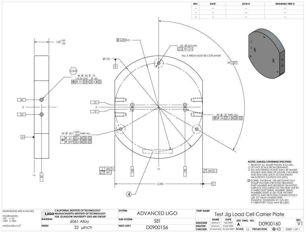
D0900160\_Test\_Jig\_Load\_Cell\_Carrier\_Plate, PART PDM REV: X-007, DRAWING PDM REV: X-004
