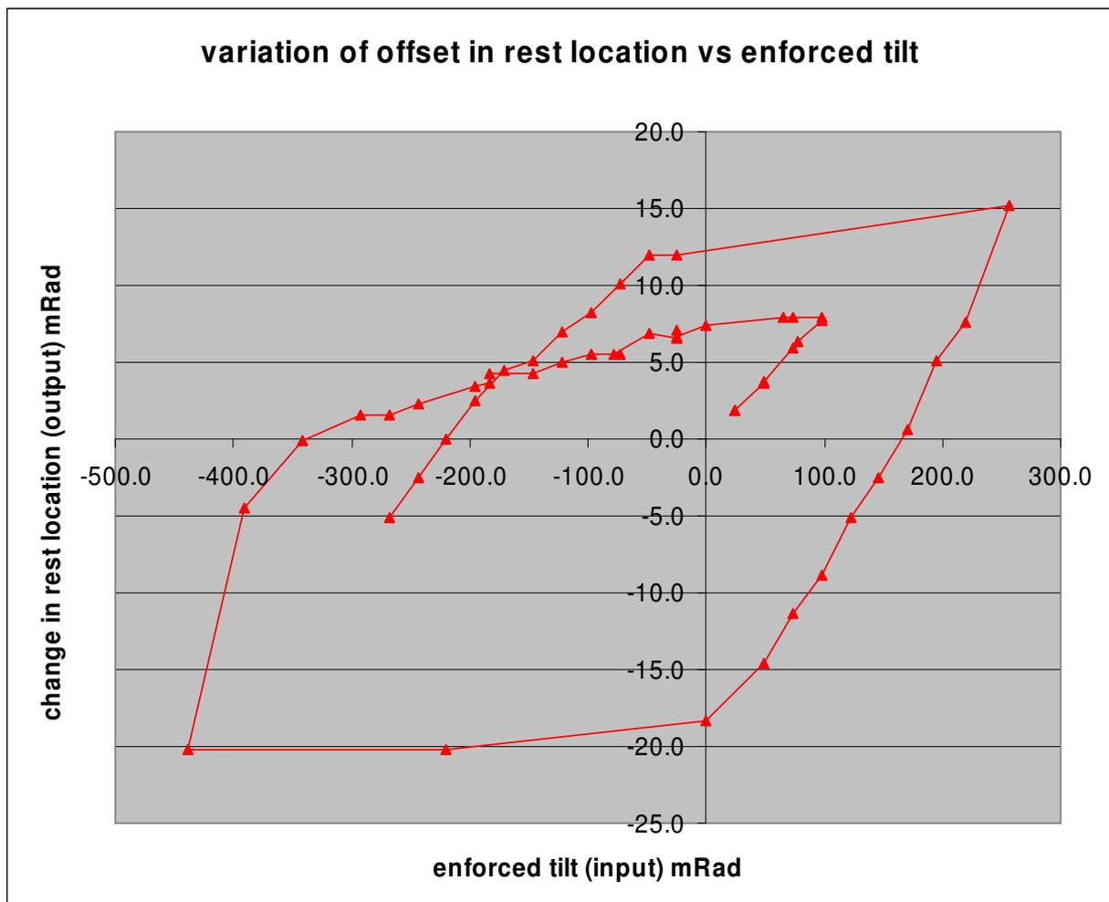
The behaviour is clearly hysteretic. We did not control of the size of the loop (we changed loading direction when we ran out space on the particular scale we were using to measure input or output, and we didn't see the full graph until we had finished!)
