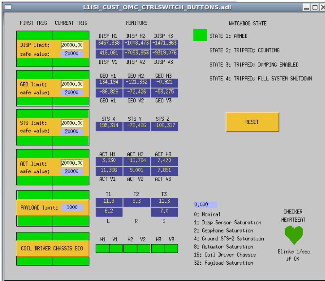
Figure 1. Watchdog screen. The checker heartbeat is in the lower right, and blinks between dark grey and green 1/sec if the checker script is running. The watchdog now watches 6 sets of inputs: the feedback displacement sensors, the feedback geophones, the floor-mounted STS-2 used for sensor correction, the actuator drive signals, the OMC watchdog, and the over-temperature monitor for the ISI coil drivers.
