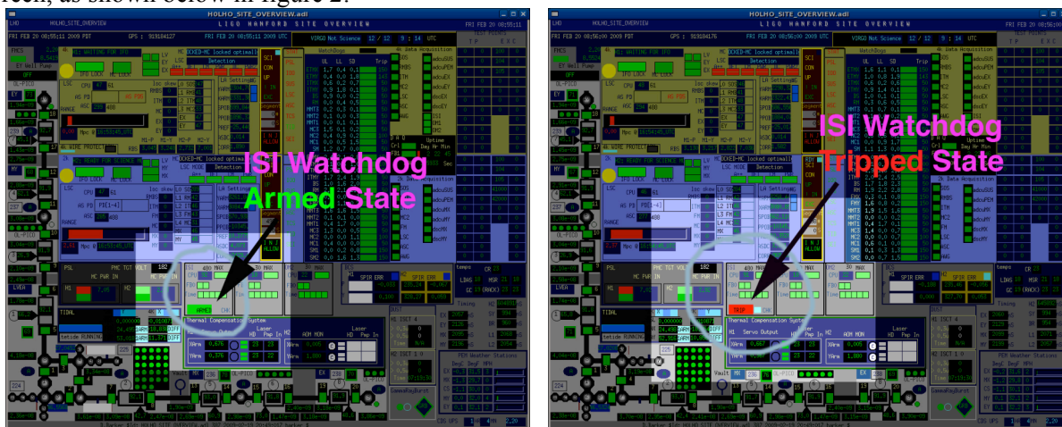
Figure 2. LHO site overview screen, showing the HAM-ISI watchdog status.
