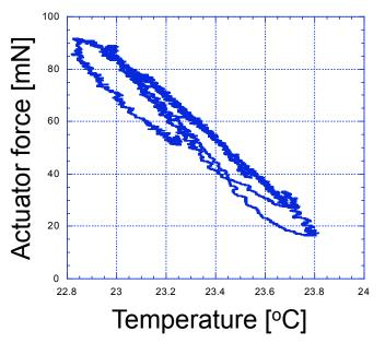
Hysteresis <u>does not</u> originate from the filter macroscopic movement **but from a microscopic dynamics** inside the
