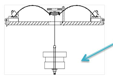
The GAS filter consists of a set of radially-arranged Maraging blades, clamped at the base to a common frame ring.
