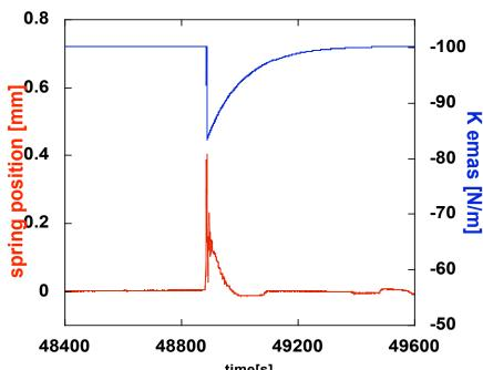
Explanation: The restoring force of the crystal lattice is nulled by the GAS and EMAS mechanism, the system is kept stable only through the restoring force provided by entangled dislocations.
