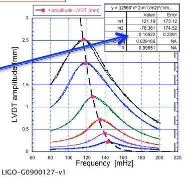
Cross checking it in the time domain by studying ring-down measurements, again the best fit
