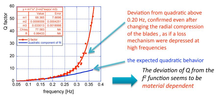
The increase of the Q-factor implies reduced losses at higher frequencies: explainable if the dissipation process needs a longer time to develop. If the system is slow enough, a limit loss level is reached, corresponding to an hysteretic regime in which dislocation avalanches can completely mobilize TIME INDEPENDENT DISSIPATION
