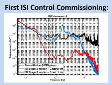
Isolation performances measured on the BSC-ISI on November 2008. The change from black to blue shows the passive isolation provided by the ISI. Blue to Red shows the active isolation. On these preliminary results the control provided isolation from 0.25Hz to 12Hz. The target for the next control commissioning is 0.1Hz to 20Hz. Black to Red shows the total isolation.
