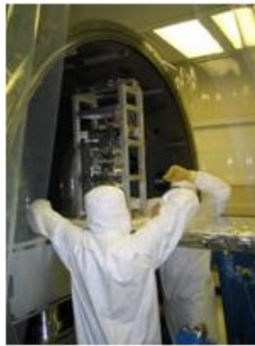
Figure 7 Left and middle: prototype modecleaner mirror triple suspension being bench tested and being installed for further test at the LASTI facility. Right: Longitudinal transfer function top mass drive to top mass position for modecleaner -green (damping off, red (damping on), blue: MATLAB model
