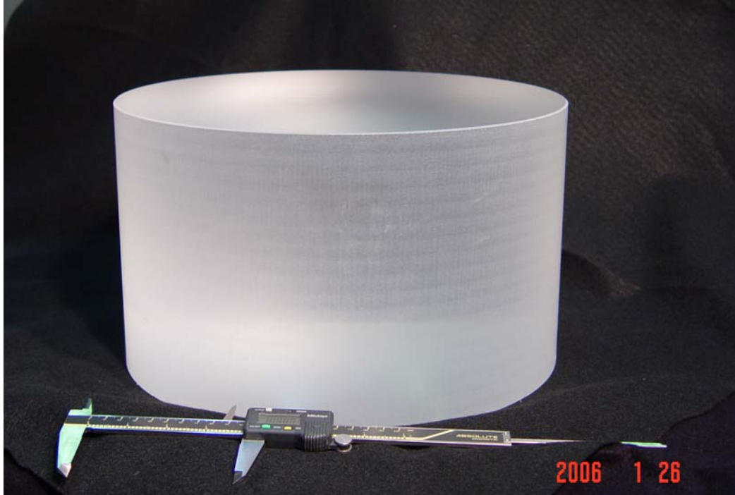
Figure 14 40kg Input test mass blank, supplied by University of Glasgow.
