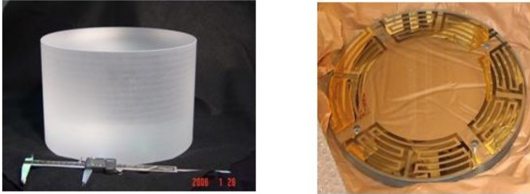
Figure 6 Left: full-size silica test mass (unpolished) procured with UK funding. Right: gold coated glass plate for testing electrostatic actuation in the controls prototype quadruple suspension
