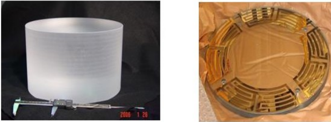
Figure 7 Left: full-size silica test mass (unpolished) procured with UK funding. Right: gold coated glass plate for testing electrostatic actuation in the controls prototype quadruple suspension
