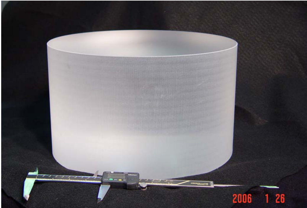
Figure 15 40kg Input test mass blank, supplied by University of Glasgow.
