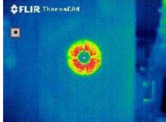
Figure 16 An initial LIGO thermal compensation pattern.
