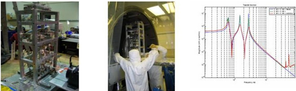
Figure 8 Left and middle: prototype modecleaner mirror triple suspension being bench tested and being installed for further test at the LASTI facility. Right: Longitudinal transfer function top mass drive to top mass position for modecleaner -green (damping off, red (damping on), blue: MATLAB model
