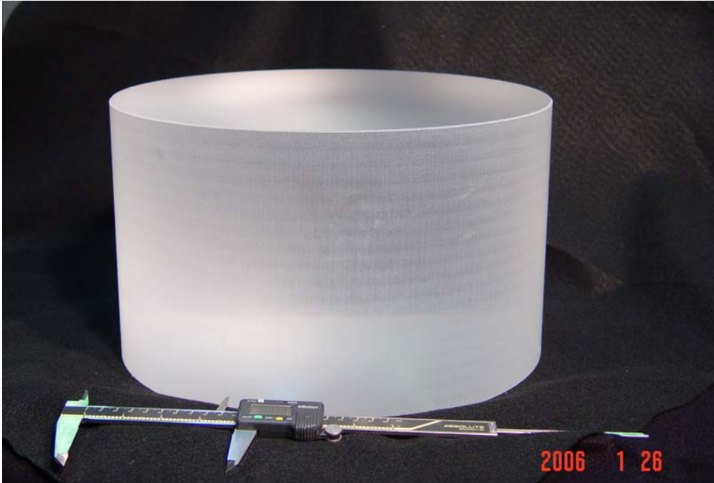
Figure 13 40kg Input test mass blank, supplied by University of Glasgow.
