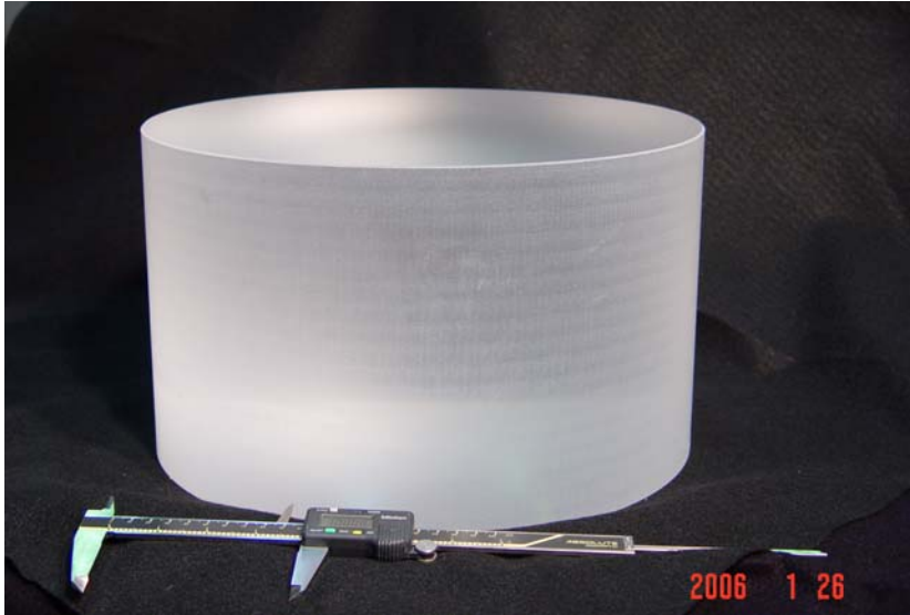
Figure 16 40kg Input test mass blank, supplied by University of Glasgow.
