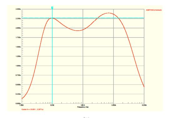
As can be seen from the plot, the noise at 10 Hz at the monitor output should be approximately  $2.3 \text{uV}/\sqrt{\text{Hz}}$ . In the table below, record the output noise at 10 Hz. The inputs to the channel under test should be tied to circuit ground and relay K3 energized relays K4 and K5 not energized (Low Noise
