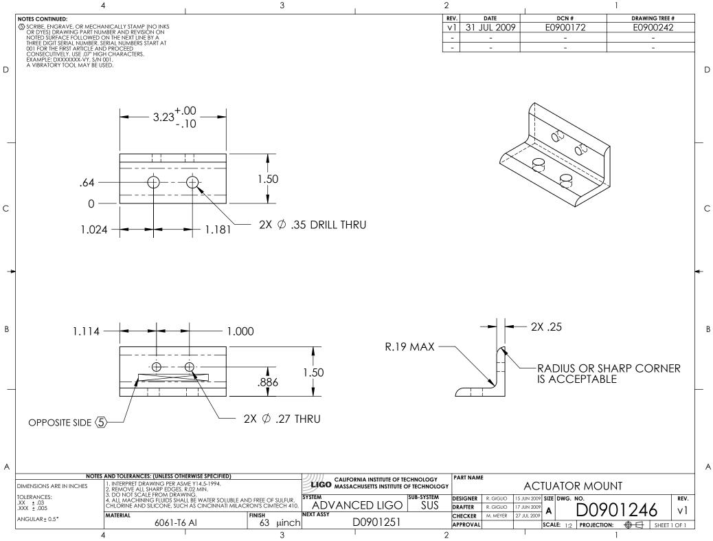
D0901246 AdvLIGO SUS Blade Test Stand Actuator Mount, PART PDM REV: X-008, DRAWING PDM REV: X-009
