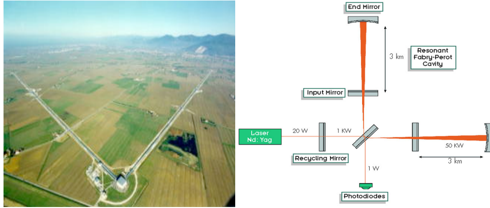
Figure 2.5: Picture and schematic of the VIRGO interferometer, Cascina.
