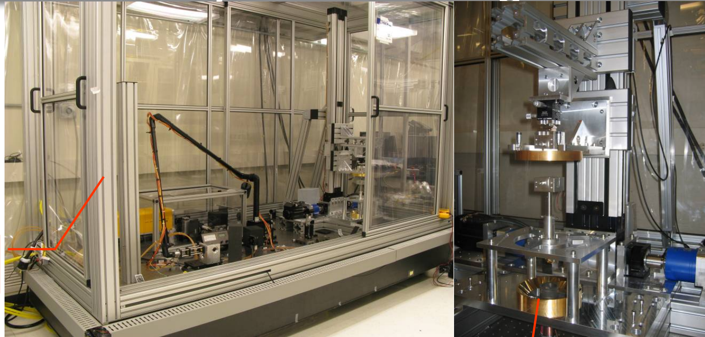
Close-up of the conical mirrors for fibre pulling
