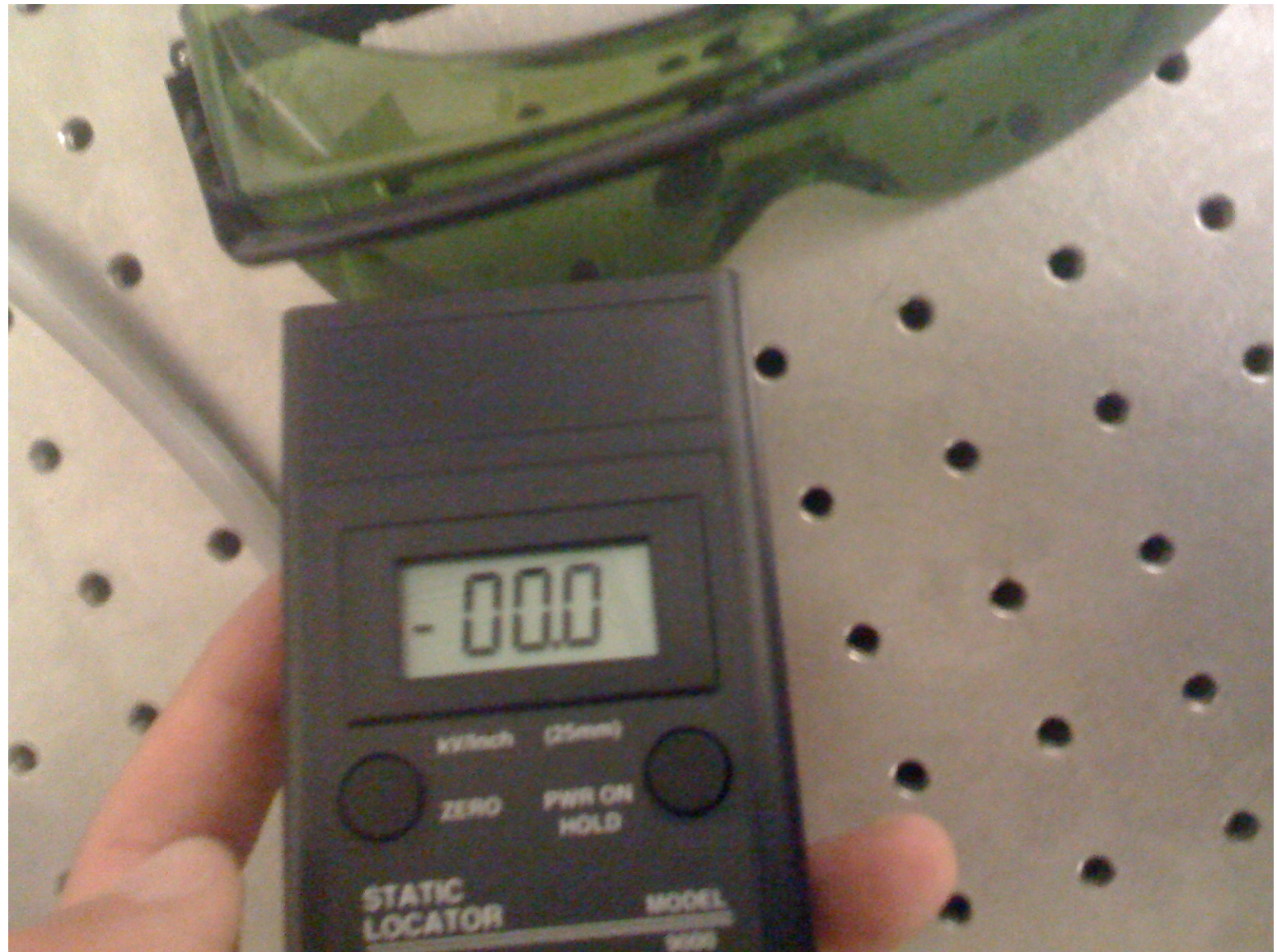
Measure the charge at the surface of an insulator (Polycarbonate LEP Goggles).
