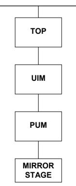
FIG 1 The LIGO Quad suspension.
