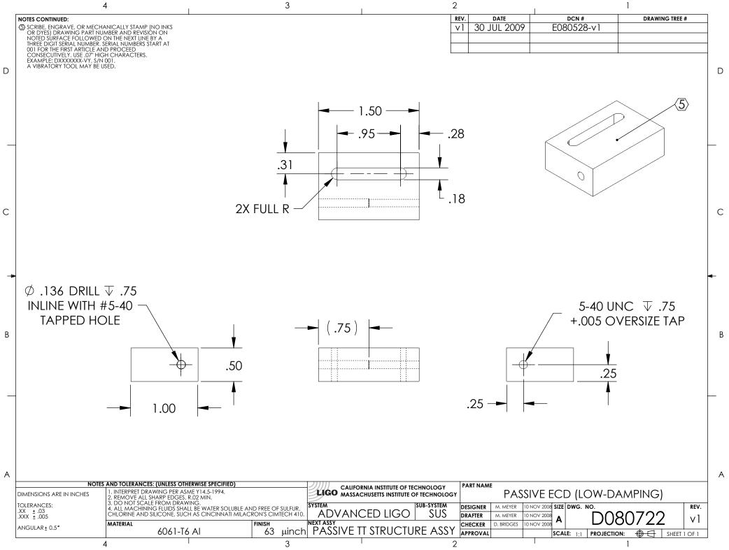
D080722\_AdLIGO\_SUS\_TT\_Passive\_ECD\_Low-Damping, PART PDM REV: X-001, DRAWING PDM REV: X-000
