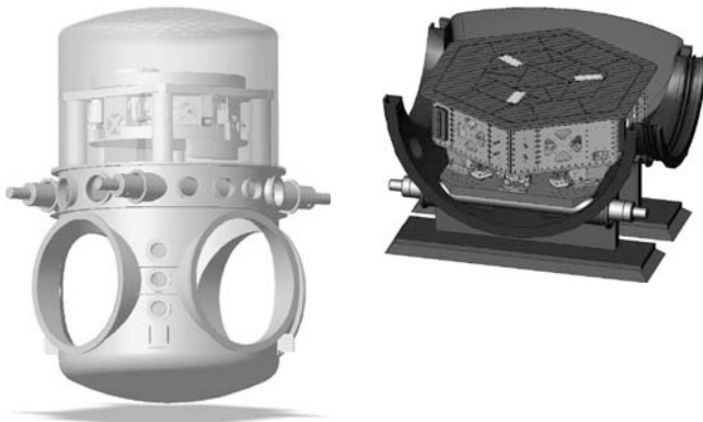
Figure 5. Computer-aided design renderings of the isolation platforms for the BSC (left-hand side) and HAM chamber (right-hand side). The top of the BSC has been rendered transparent to show the isolation platform. The doors and external supports of the BSC are not shown. The HAM platform is shown in a sectioned HAM chamber.
