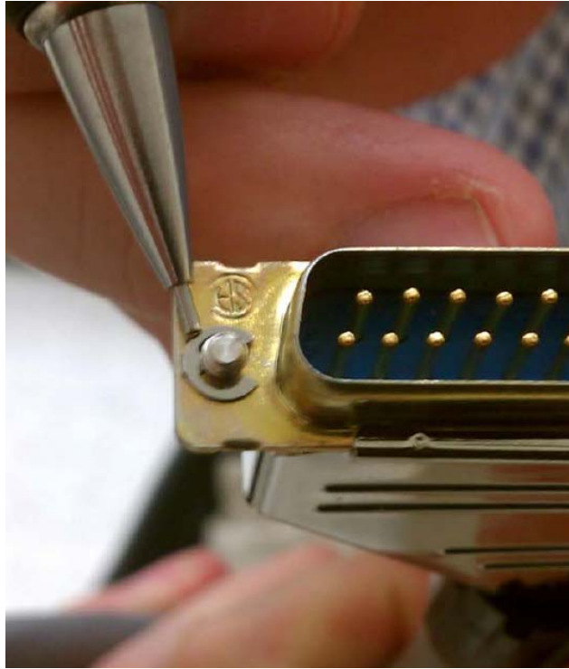
Figure 11, THIS IS THE WRONG PLACE FOR THE E-CLIP
