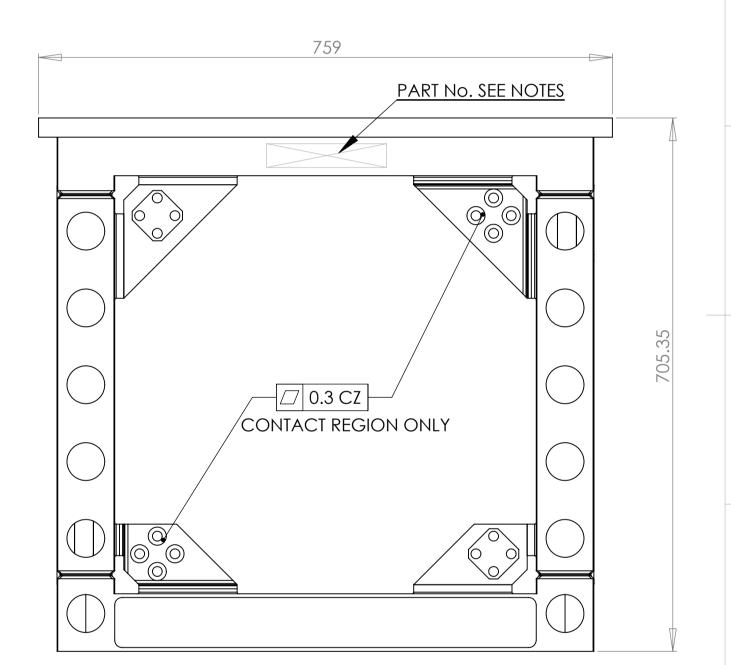
DRAWING SHOWING FULL UPPER STRUCTURE WELDMENT DRAWING NOT INTENDED FOR MANUFACTURE DETAIL OF WELD PREPS, TOOLING RADS, FAB STEPS EXCLUDED
