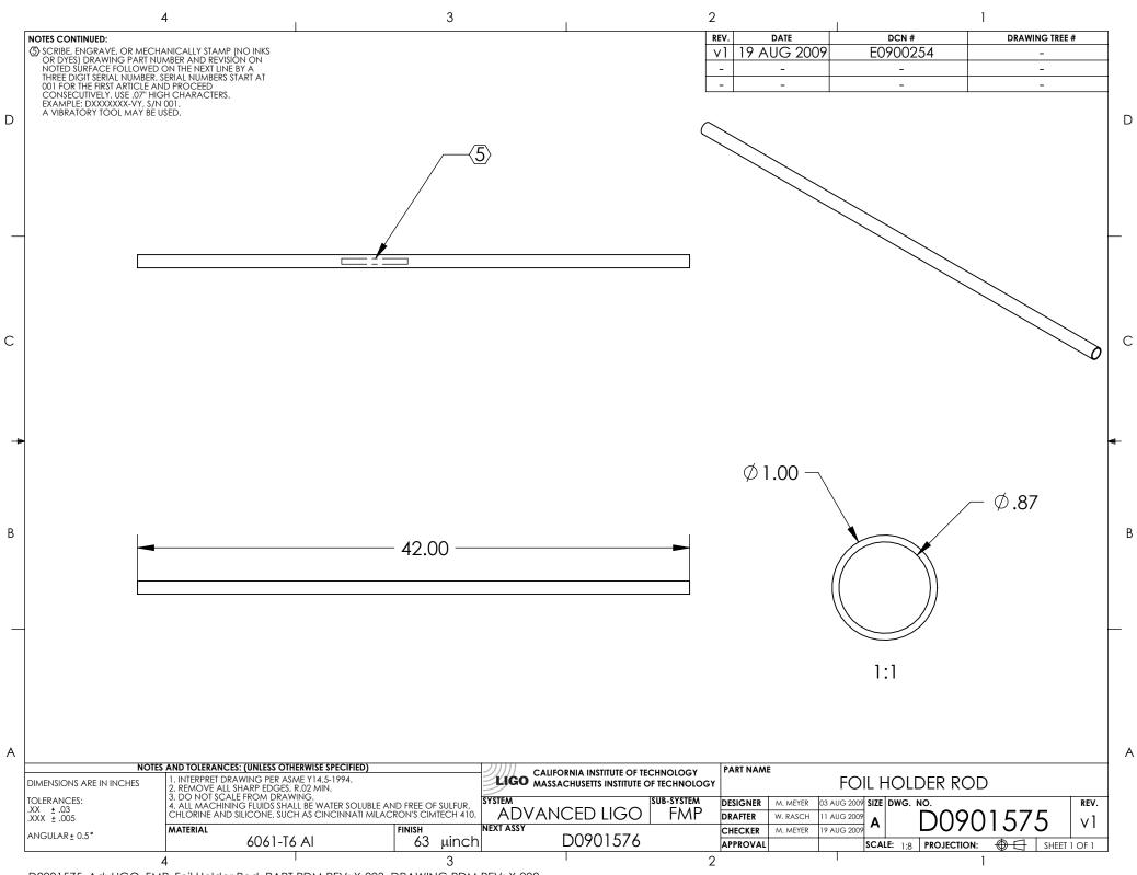
D0901575\_AdvLIGO\_FMP\_Foil Holder Rod, PART PDM REV: X-003, DRAWING PDM REV: X-002
