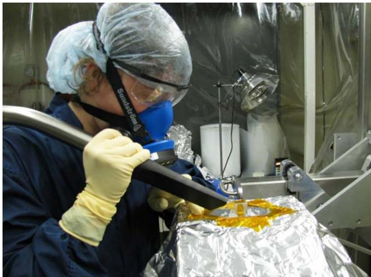
**Figure 3: Wearing protective goggles and respiratory mask with P3 dust filters**
