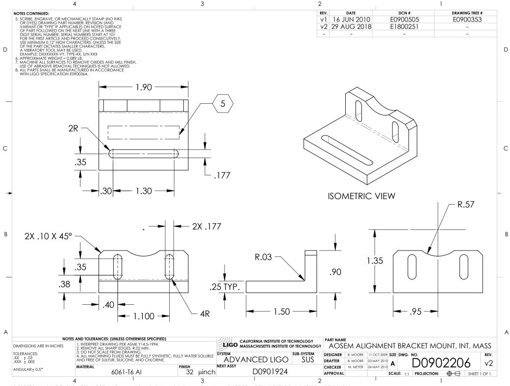
D0902206\_AdvLIGO\_SUS\_HSTS\_AOSEM Alignment Bracket Mount, Intermediate Mass, PART PDM REV: X-017, DRAWING PDM REV: X-011
