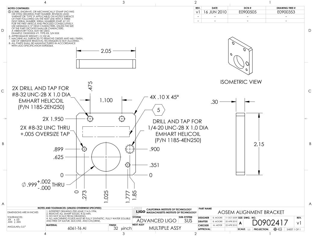
D0902417\_AdvLIGO\_SUS\_HSTS\_AOSEM Alignment Bracket, Test Mass, PART PDM REV: X-006, DRAWING PDM REV: X-004
