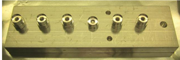
Fig 61: Heating Fixture with Holders
