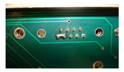
There should be a diode soldered under the negative Voltage Regulator (U2) (ECR E1300535-v1)
