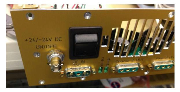
Plug the four crimp terminals onto the back panel switch. For uniformity, I plug the input power onto the bottom pins (positive (red) on the left, as viewed from the top, and negative (green) on the right. I then plug the outward bound power onto the top two pins, with the colors on the same sides as the bottom two:
