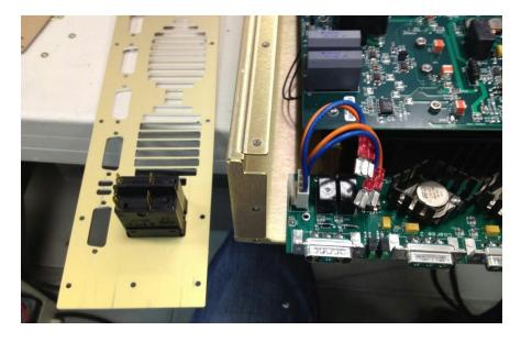
Unscrew the Fine/Coarse 2 fan and electronics module by removing the three screws underneath:
