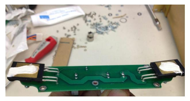
Using four 4-40 nuts, attach the boards to the chassis. Be sure that the pressure screws that push the FETs against the wall of the enclosure are fully backed out. Once the nuts are tight, you can push the FETs against the side wall, and finger-tighten their associated pressure screw:
