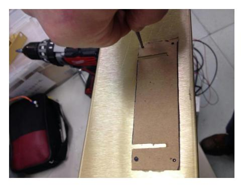
Drill these holes out with a 7/64" or #36 drill bit:
