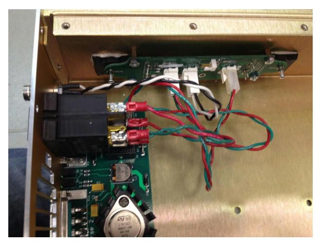
Now, to fix the two other manufacturing issues, if they're present. At this stage, power up the board, and see if all the surface mount leds light up. If the +15V LEDs do not light, they are in backwards, and need to be turned around:
