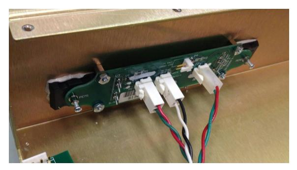
Remove the switch from the old panel, and place it into the new rear panel. Also attach the Watchdog BNC, and put the back panel back together, remembering to install the necessary split washers:
