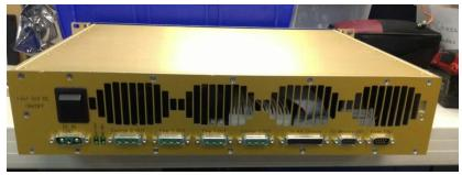
In addition to installing the Driver Cutoff circuit, we should also take care of some manufacturing issues while we have the box open, and check to see if the back boards are up to date. The first of these is the absence of the locking washers under the Dsub jackscrews:
