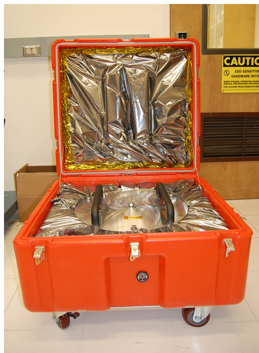
Figure 5: Proper orientation of the FM/BS container top handles and foam. The foam fits between the top handles.
