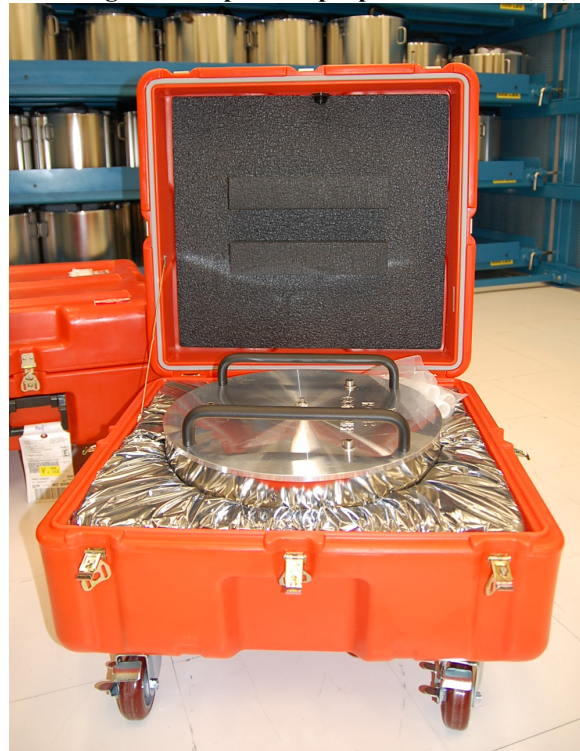
Figure 3: Proper orientation of shipping case foam and top handles on ITM, CP and R cases. Note the two foam rectangles that fit between the top handles of the optic container.
