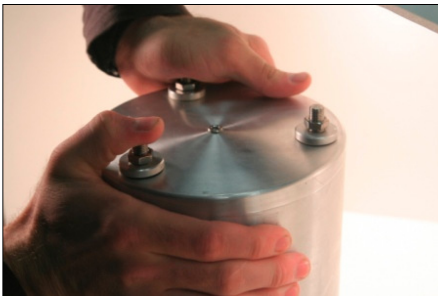
Figure 9: Push down on the studs while gripping and pulling up on the can until...
