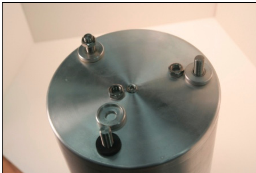
Figure 11: Next remove the nuts, cap washers, and grommets and set them aside for reassembly later
