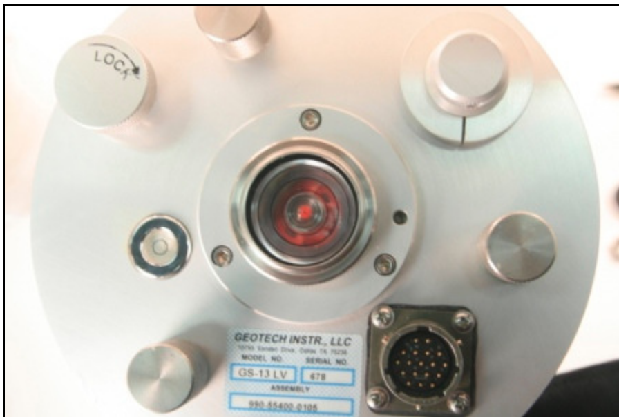
Figure 50: Unlock the proof mass and look at the red indicator - it should fill the center ring completely
