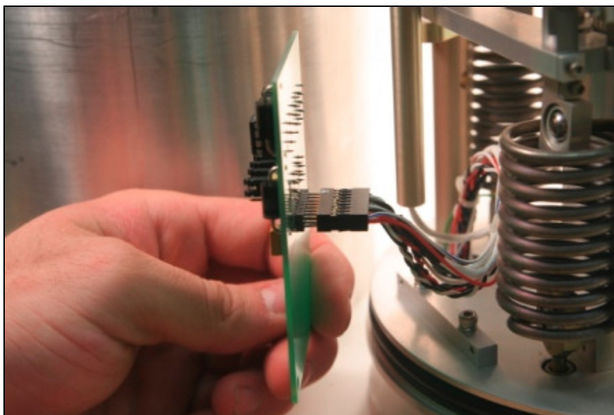
Figure 20: Tuck the wires back in making sure that the wires do not contact offload springs, cantilevers, or flexures
