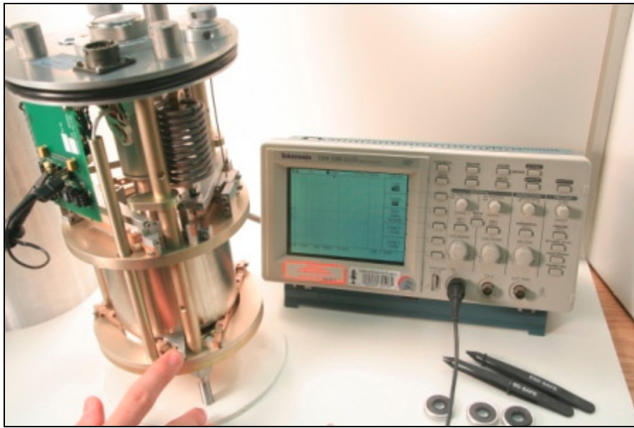
Figure 53: Take a ring-down by holding the mass down against its stop and releasing it
