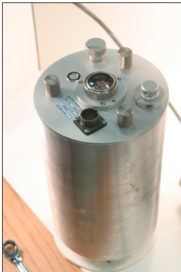
Figure 65: Completed GS-13 flexure retrofit ready for podding in aLIGO
