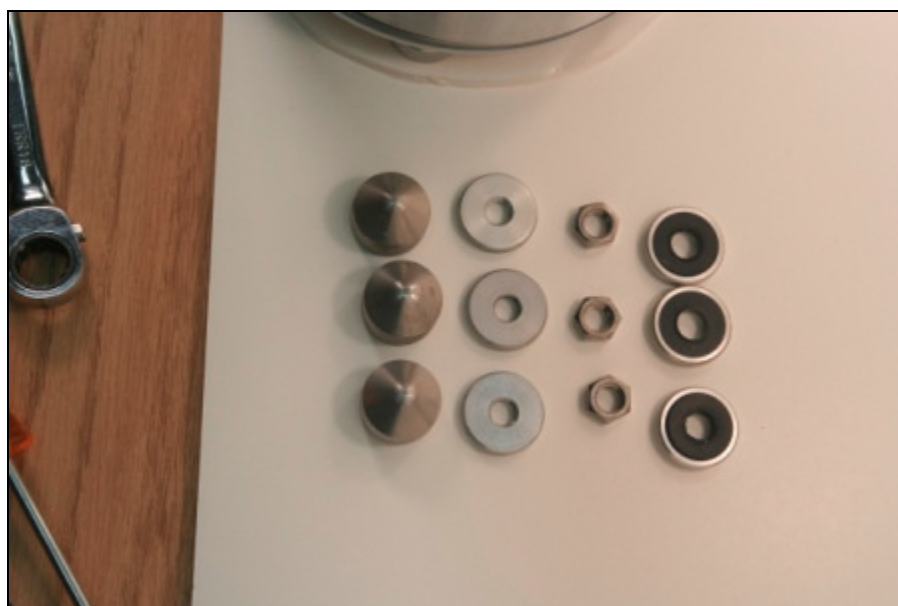
Figure 12: Removed hardware for can removal
