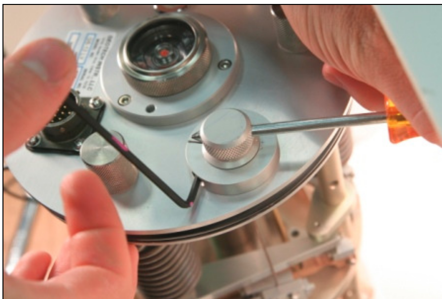
Figure 55: To raise the natural frequency loosen the lock collar with the 7/64 hex wrench and turn the knob counterclockwise to increase the frequency
