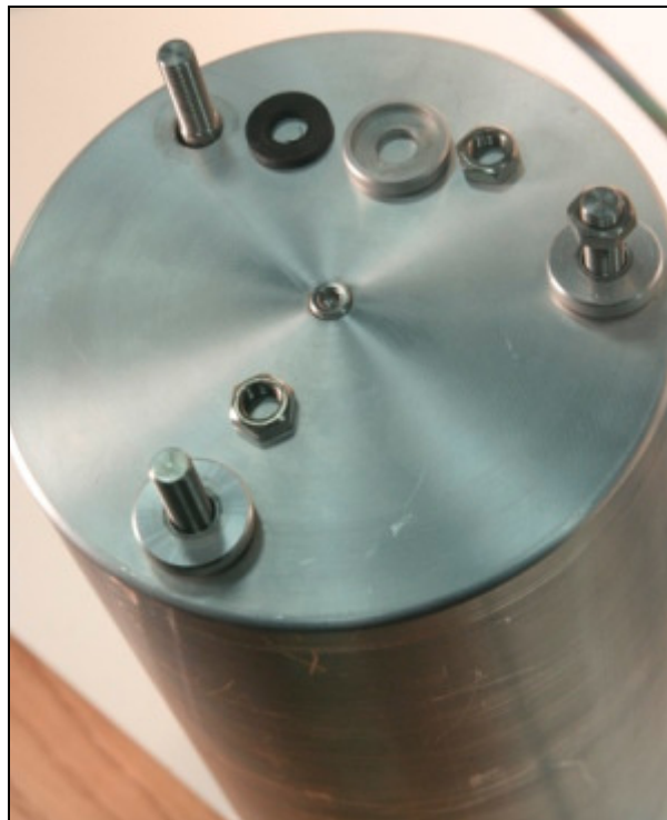
Figure 62: Install the grommet, cap, and nut on the studs. Tighten with the 9/16 wrench
