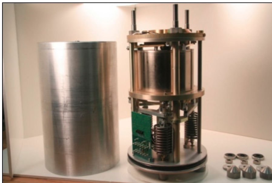
Figure 14: GS-13 with can removed
