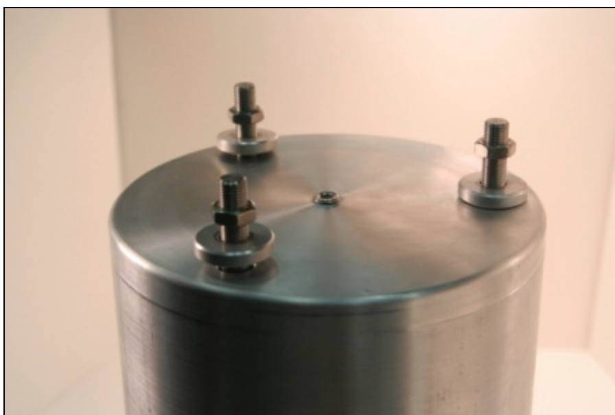
Figure 8: Slide the aluminum washer cap and rubber grommet up slightly on each stud
