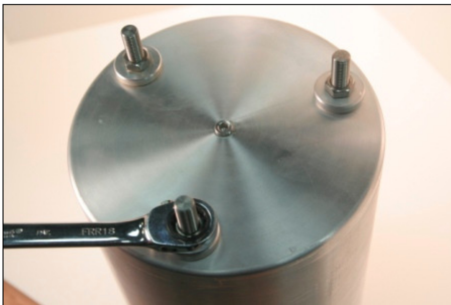
Figure 7: Using the 9/16 combination wrench, loosen the three nuts to about halfway up the stud
