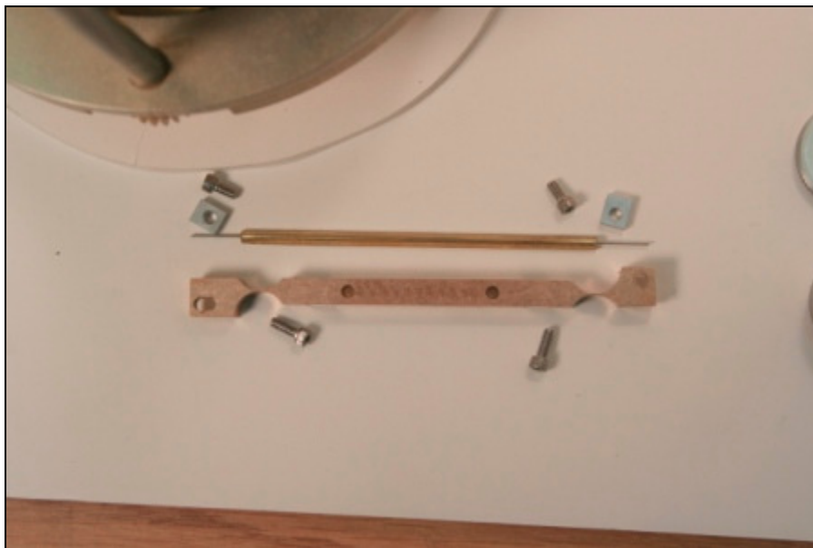
Figure 31: The removed delta rod, SHCS, and plates (top) will not be reused, the new flexure and 4-40 x 3/8 in. SHCS bottom will be installed
