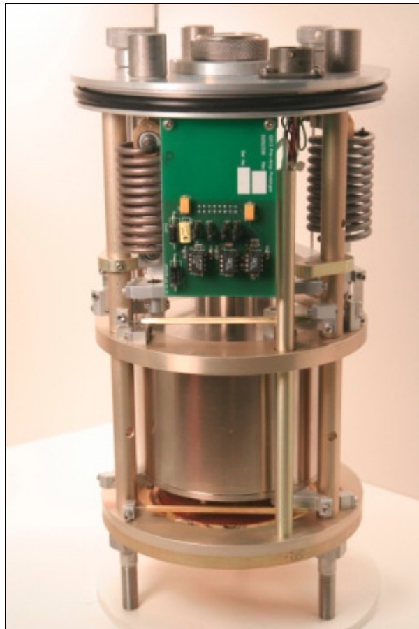
Figure 23: Turn the GS-13 over and set it on its studs
