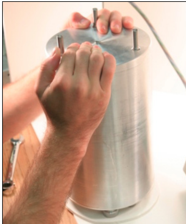
Figure 61: A fairly large downward force is required to slip the cover over the o-ring
