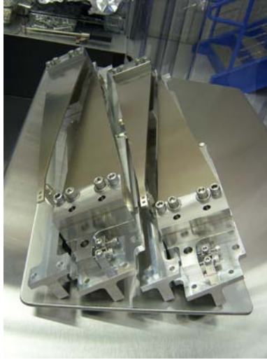
Figure 4 TS Blade Cartridge Assembly D060324
