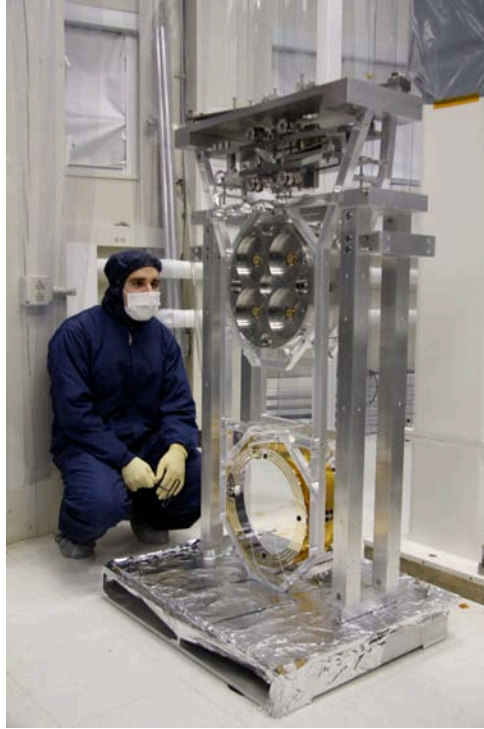
Figure 22 Brett Shapiro Inspecting alignment of Reaction Chain LASTI Quad
