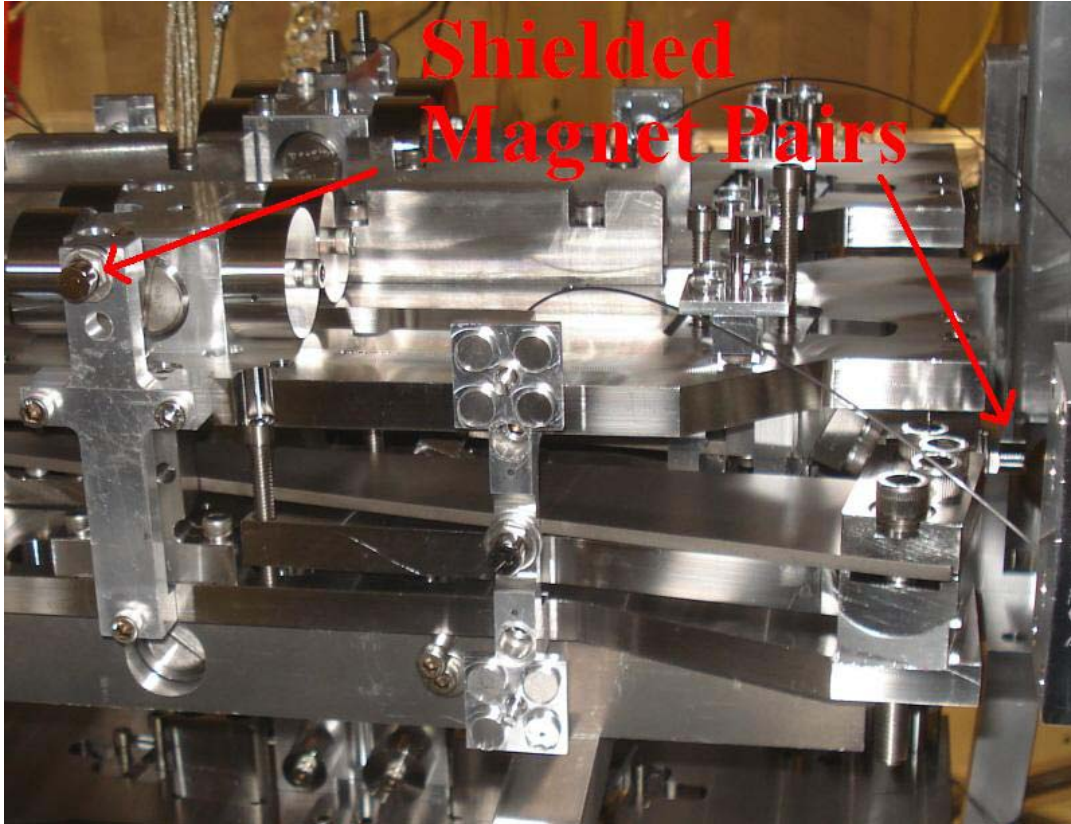
Figure 11 This photograph shows the locations of the shielded magnet pairs around the top mass. In LASTI notation these are the magnets belonging to the 'Side' and 'Face 1' OSEMs. The UI mass OSEMs also have shielded magnet pairs.
