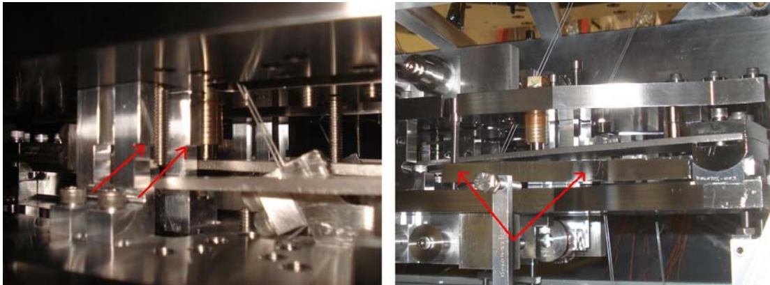
Figure 14 The left photograph shows the vertical blade tip reference points indicated by the red arrows. The arrows are pointing to a lip on one of the two upright U shaped aluminum parts that arch over the blade tip. For the UI mass, there should be 15 mm between the top of the blade and that lip when the round masses are suspended below. There should also be 5 mm of clearance on either side between the tip and these U shaped parts [3]. The right photograph shows the adjusting arm for the blade tip height. Just above the left red arrow is a long upright 1 4-20 bolt. Turning this bolt will adjust the angle at which the blade leaves its clamp, allowing the tip to move up and down. It may be necessary to slightly loosen the two outer bolts in the clamp (the ones closest to and furthest from the opposing chain). The UI spring clamp bolts should be torqued back to 100 in-lbs (8.3 ft-lbs, 11.3 Nm) [6]. The top mass springs are referenced and adjusted in a similar way. The top mass clamp bolts get torqued to 330 in-lbs (27.5 ft-lbs, 37.3 Nm) [6].
