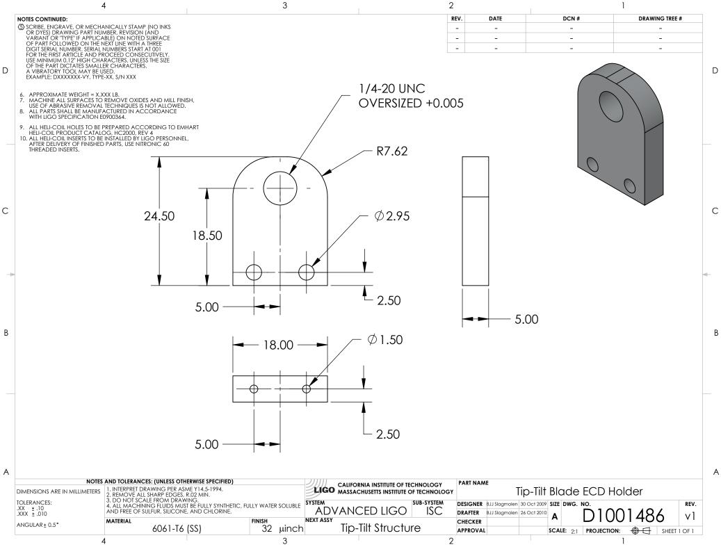
D1001486\_v1\_Tip-Til\_Blade\_ECD\_Holder, PART PDM REV: , DRAWING PDM REV:
