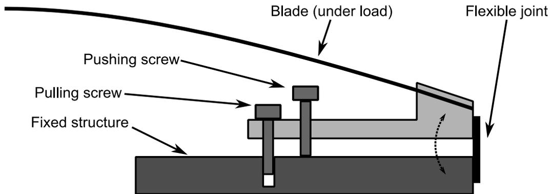
**Figure 4. Sketch of the blade adjusting mechanism. The pull and pushing screws force the flexible joint to bend, thus modifying angle of the blade.**
