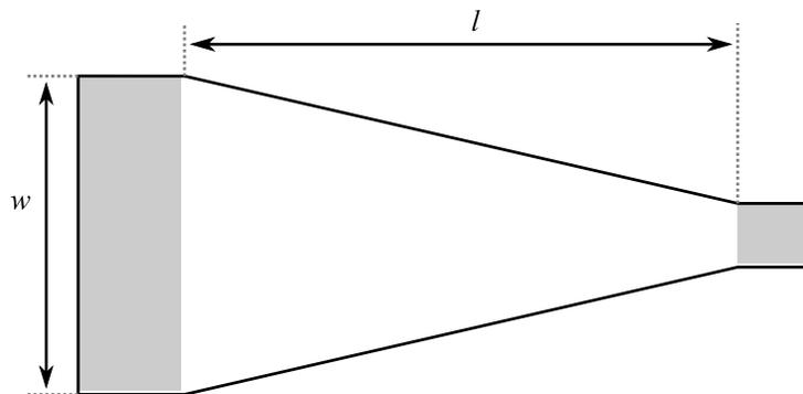
**Figure 3. The approximate shape of one of the two blades used for vertical isolation.  $l$  has been chosen to be 76.8 mm, while  $w$  is 40.6 mm.**
