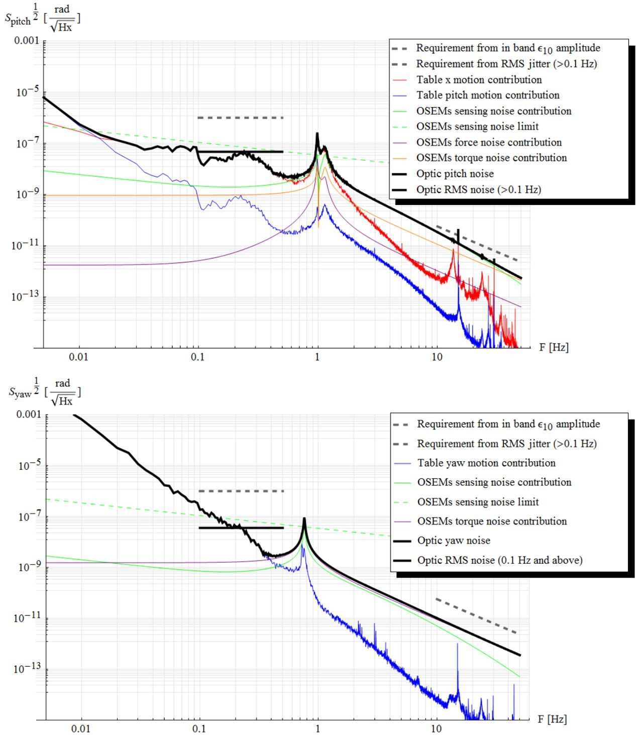
**Figure 8. Overall closed loop HAM Aux pitch and yaw noise calculated using the Mathematica model mentioned in the text (see [LIGO-T1000339](#)). Contributions from individual noise sources are also shown.**
