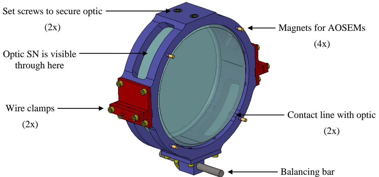
**Figure 5** The aluminum barrel that holds the optic and hosts all the mounting fixtures. Some of them are indicated in the picture.
