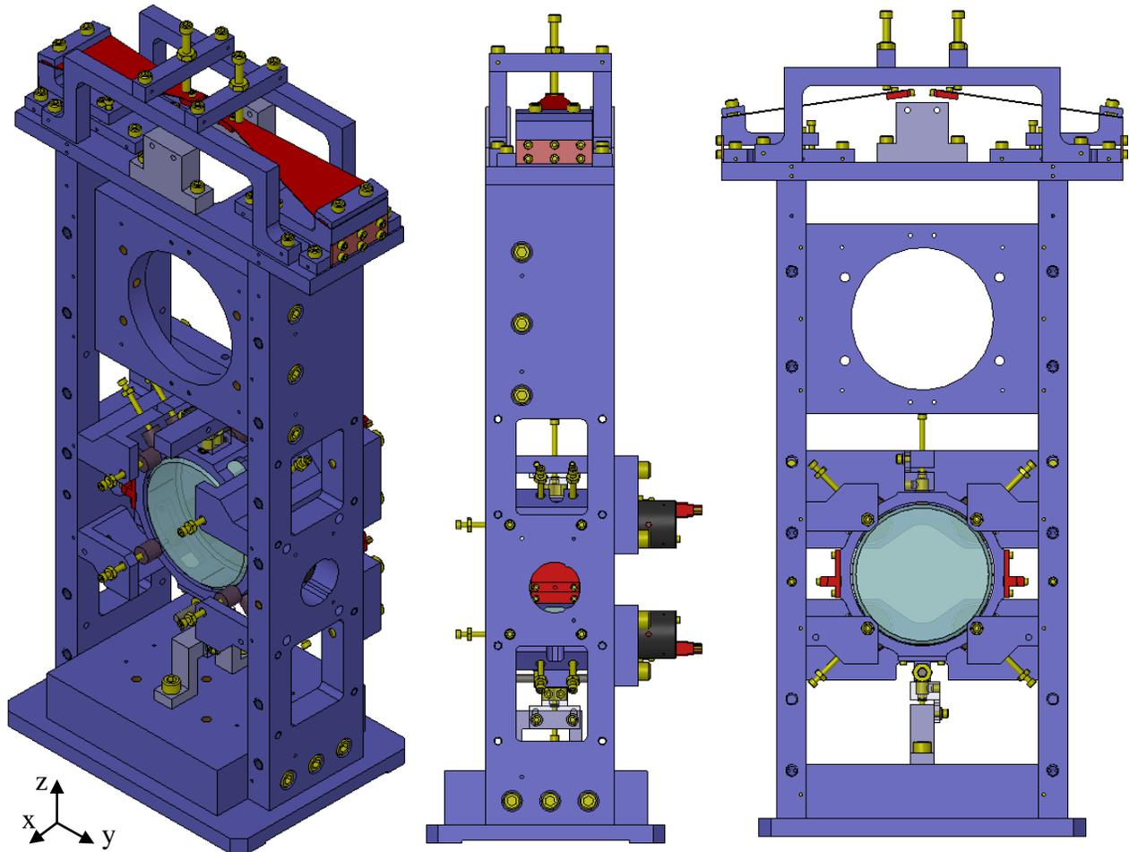
**Figure 1. SolidWorks model of the HAM Aux Suspensions. Coordinate system is taken to have the x axis coincident with optic axis, pointing from the back of the suspension (the one with the AOSEMs) towards the front of the suspension (where the HR side of the optic is), and z one in vertical, pointing upwards (see the small axes at the left of the figure).**
