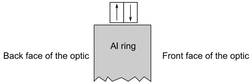
**Figure 7. A conceptual drawing showing a lateral view of how the magnets are positioned for eddy current damping. The top part of the optic holder is shown. The two white rectangles represent the two cylindrical magnets, and the arrows indicate the direction of magnetization. The magnetic field in the region of the Al ring next to the magnets is almost parallel to the optic axis, thus effectively damping the bounce, roll and y movement of the suspended assembly.**
