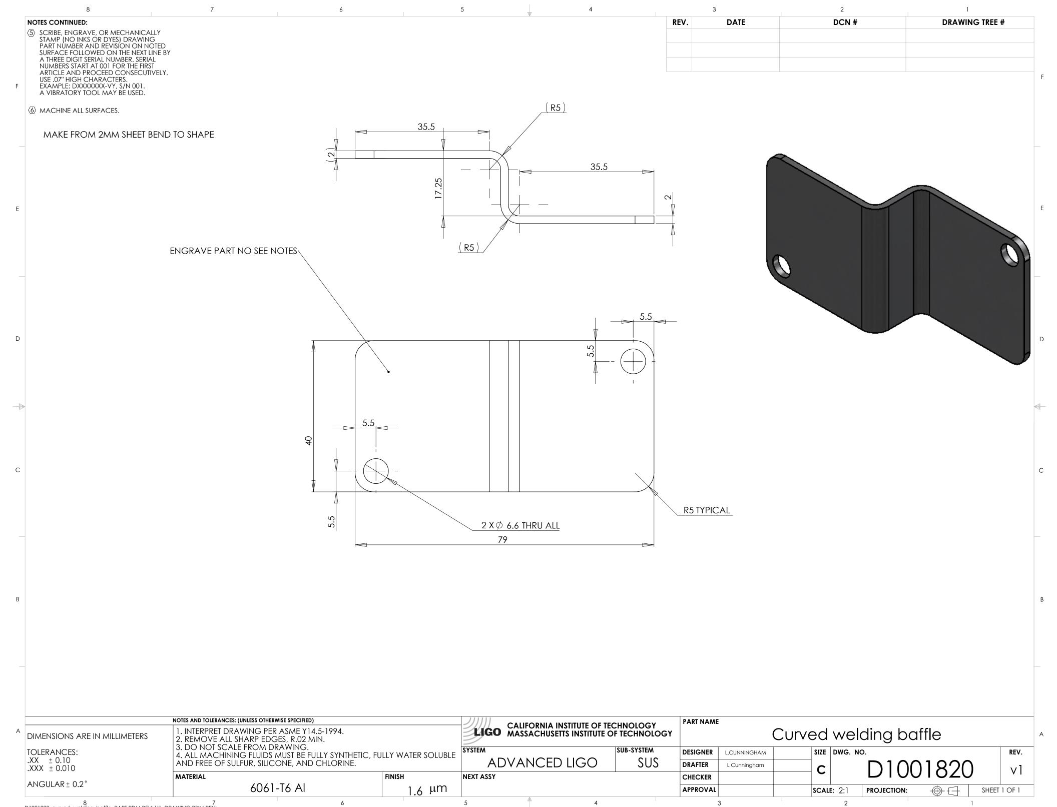
8 D1001820\_curved\_welding\_baffle, PART PDM REV: V1, DRAWING PDM REV:
