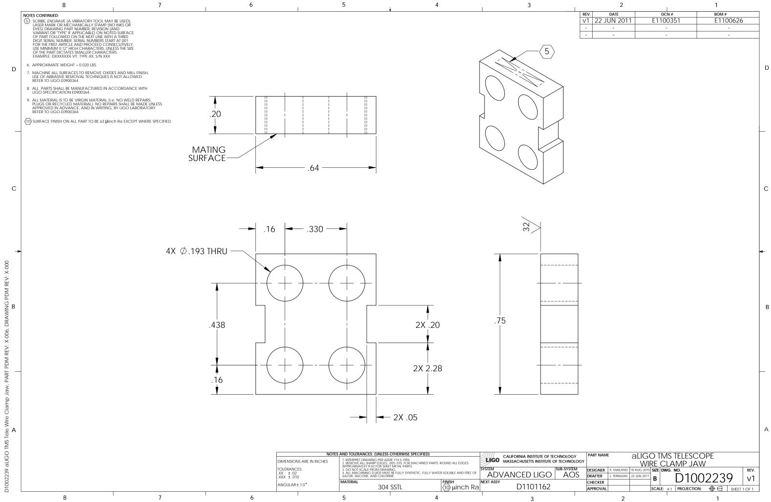
PART PDM REV: X-006, Jaw, Wire Clamp
