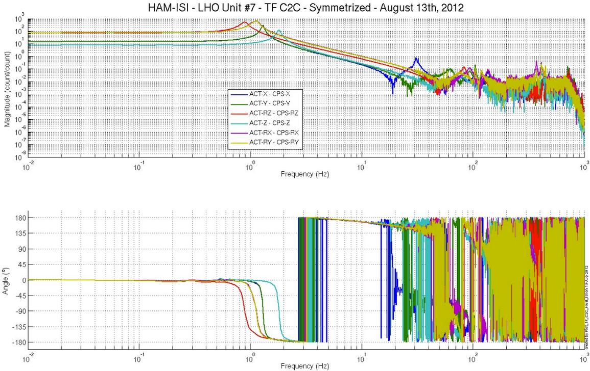
**Figure – Cartesian to Cartesian – computed - Capacitive sensors**
