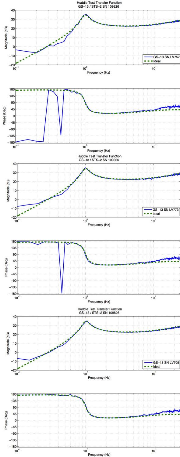
Figure - Huddle testing of Vertical GS-13 757(V1), 773(V2), and 705(V3) after aLIGO modifications
