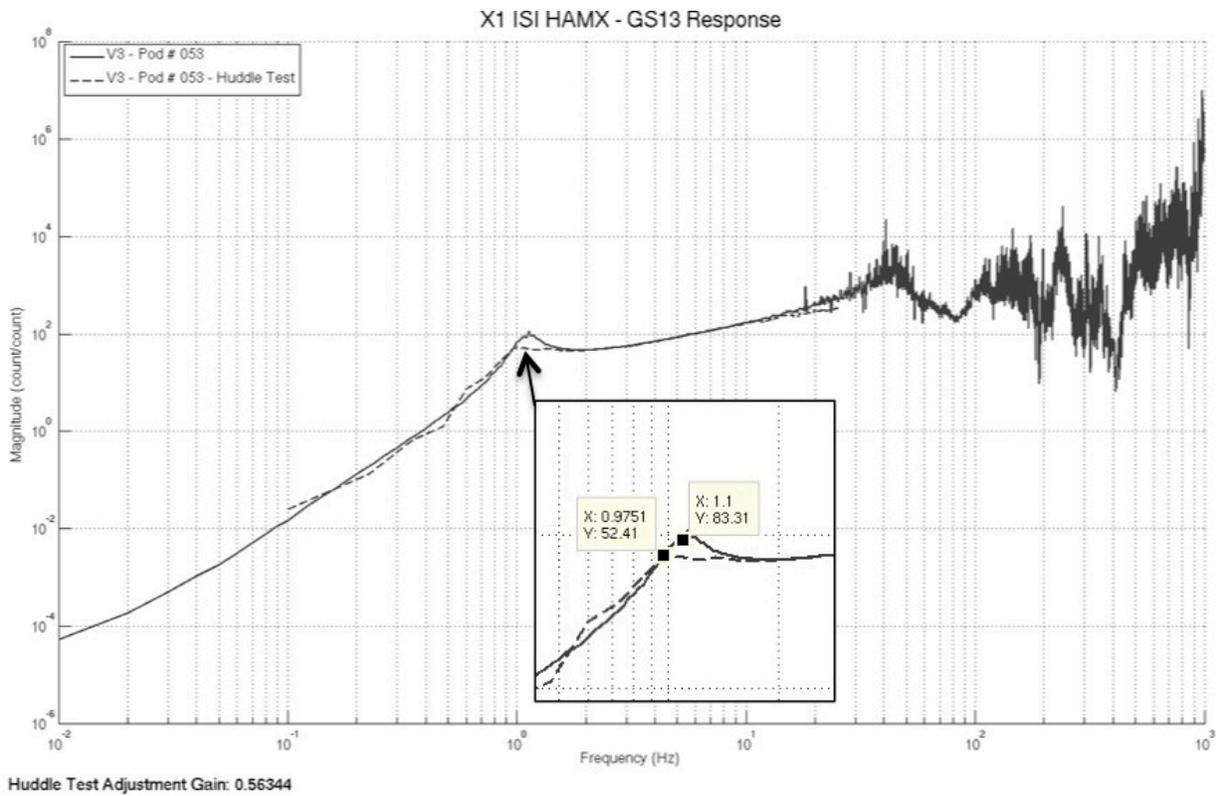
figure – GS13 extracted responses VS Huddle test responses
