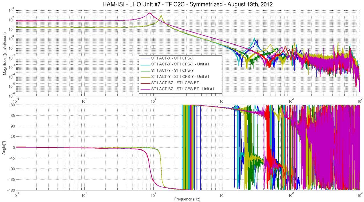
**Figure – Cartesian to Cartesian measurements, comparison with Unit #1 reference
