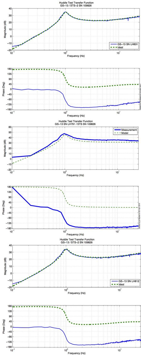
Figure - Huddle testing of Vertical GS-13 831(H1), 791(H2), and 812(H3) after aLIGO modifications
