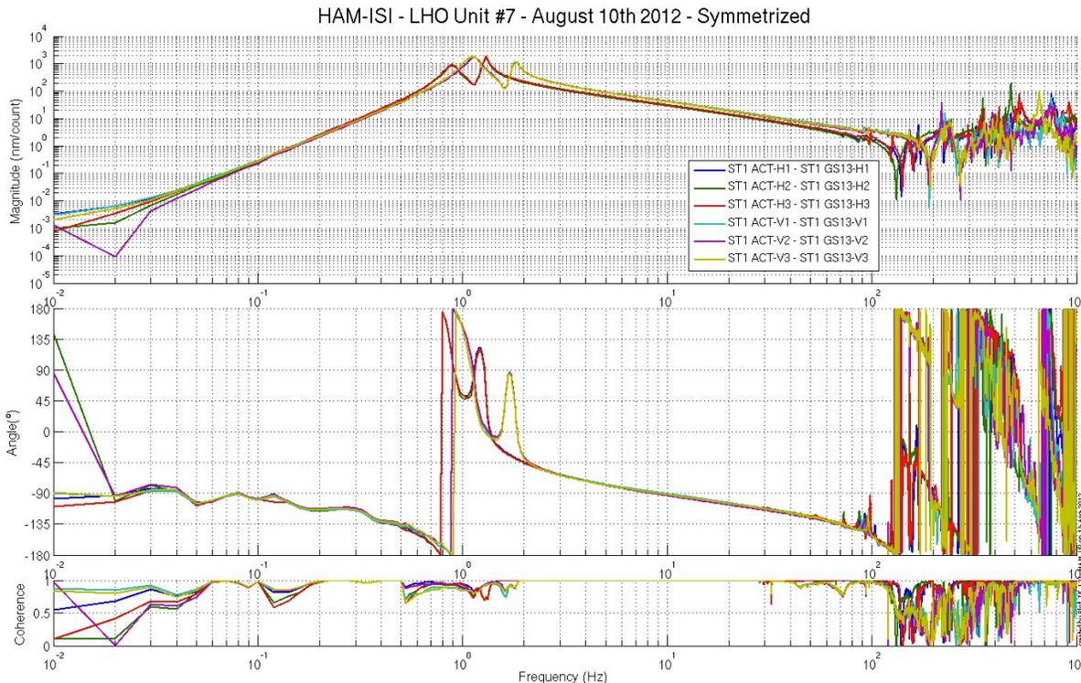
figure – Symmetrized L2L – Computed TFs – Inertial sensors
