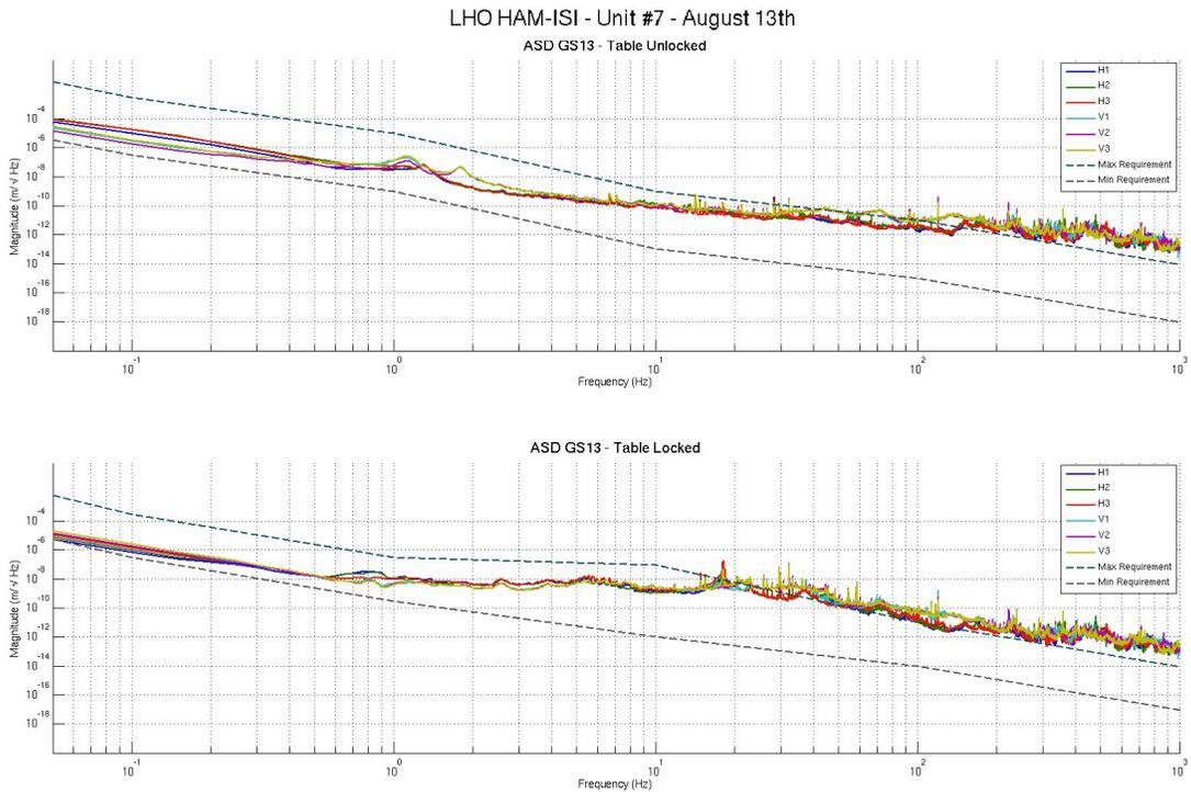
**Figure - Calibrated GS13 Power spectra**
