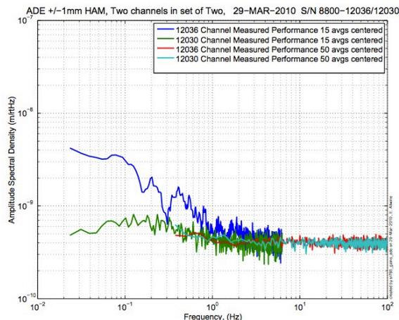
Figure - H3 and V3 sensor noise
