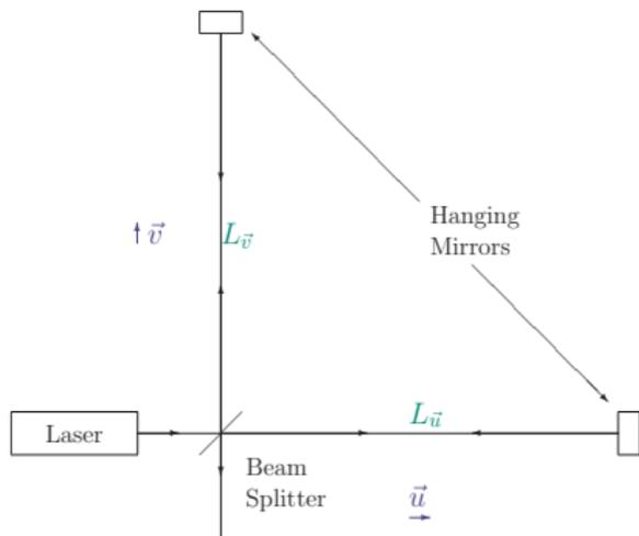
Laser interferometer measures strain  $h$ , given by
