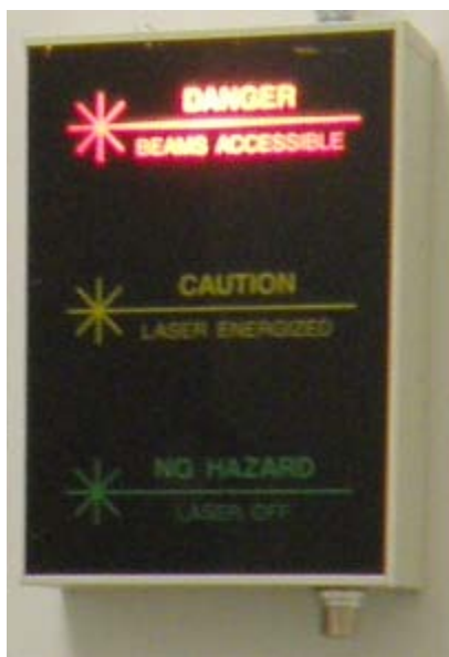
Figure 1: A typical wall mounted laser safety sign. This one shows that an area is presently in laser hazard. The status key switch (silver) can be found in the lower right of the picture. The “Caution” state is never to be used.
