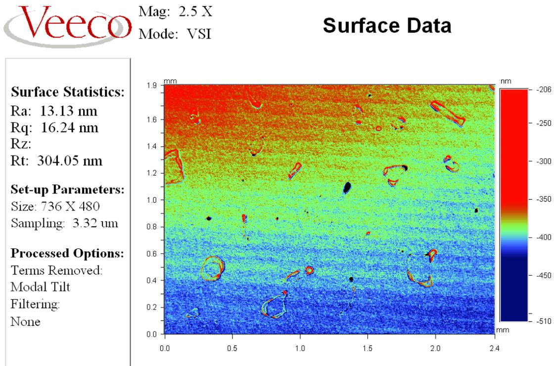
Fig3.10. Marks left behind by bubbles on the surface of a silica disc.
