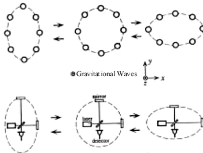
*Fig1.1. As a gravitational wave passes across the object it causes a distortion – first in one direction, then in the next – changing the shape of the object. In the same way, as it passes across the interferometer, it changes the arm-lengths. This effect could be measured by the interferometer.*
