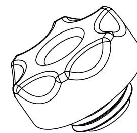
Actuator Plate Plug D020359-2A Mat'l: 6061-T6 (5) required
