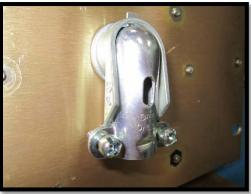
5. Insert the adjustable cam latch through the keyed hole on the lid, slide the nut over the latch and tighten.
