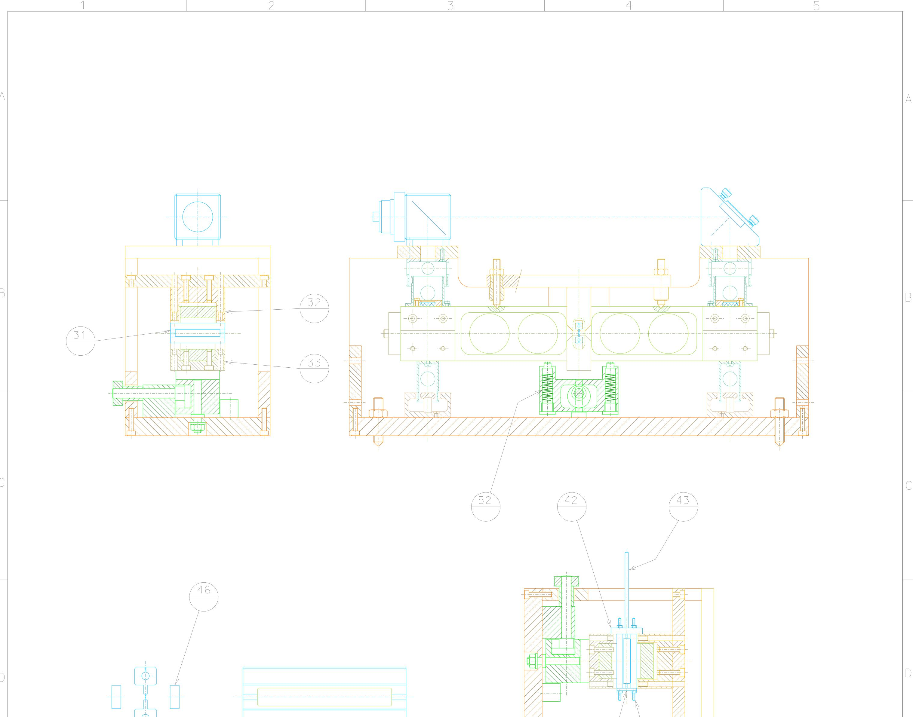
Instruction for assembly of part 31 into tiltmeter: With the balance locked, put tiltmeter on its side with part 31 still held between the two transport plates 46, screw assembly plate 42 and 44 on the side of part 31. With part 31 sitting vertically on the table, release screw holding the two parts 46 and remove them. Inspect the flex joint. Lift 31-42-44 from the center screw and lift it in position tie lock set screws in part 32. Rotate tiltmeter on its base. Release screw holding part 42-44.
