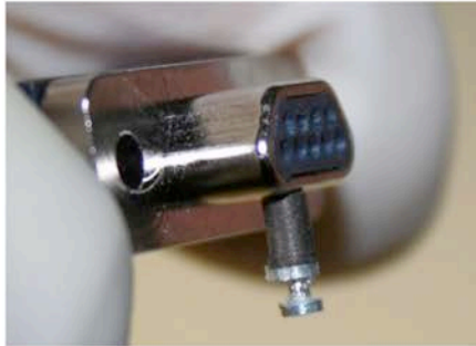
Connector (with suspended test mass magnet)
