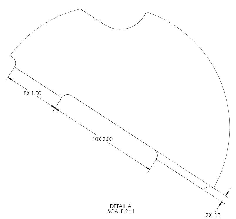
THIS PIECE IS PART OF A WELDMENT. DIMENSIONS SHOWN ARE APPROXIMATE; WELD INDUCED SHRINKAGE OR FILL AND POST WELD ANNEALING AND MACHINING CONSIDERATIONS ARE NOT INCLUDED. SEE NEXT ASSMEBLE FOR REQUIRED DIMENDIONS FOR STRUCTURE AFTER WELDING.
