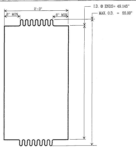
FIGURE 2 - EXPANSION JOINT DIMNSIONAL LIMITATIONS
