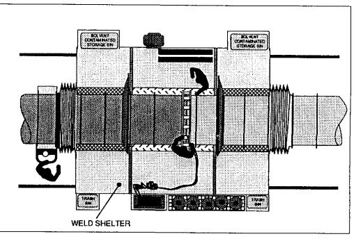
STEP #11 - REMOVE FIT-UP FIRTURE AND INSTALL
