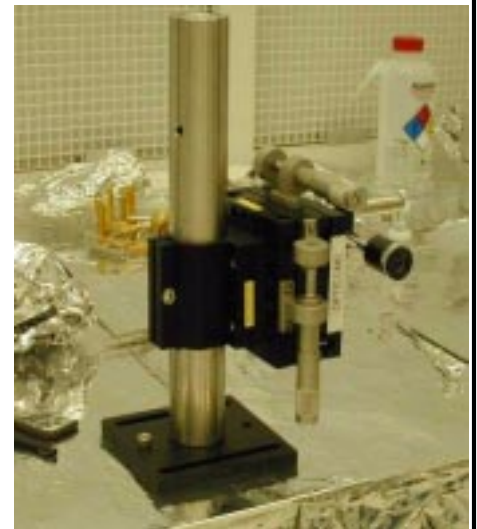
Traveling microscope, mount, and vernier adjustments
