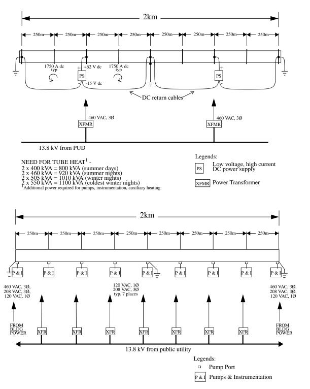
DC power supply layout (top); AC power distribution for heater jackets, pumps and instrumentation (bottom)
