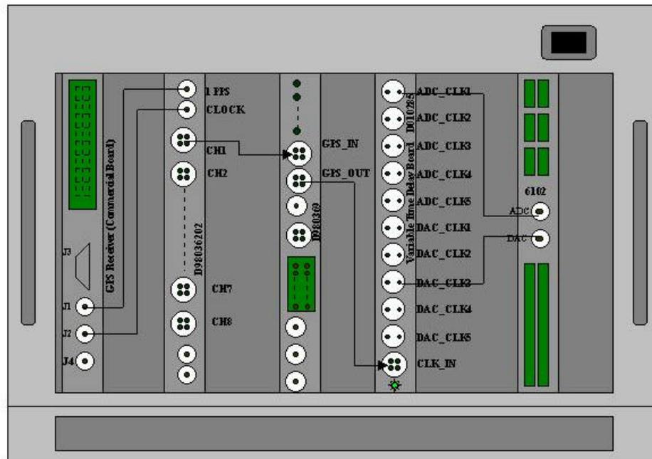
In the far left slot of the crate is a GPS receiver module developed by Brandywine Communications for the LIGO project. This module receives and decodes signals from GPS satellites and provides 1 PPS (1 pulse-per-second) and  $2^{22}$  Hz clock signals to a GPS Fanout Module (D980362-02) designed by LIGO Laboratory. The  $2^{22}$  Hz clock is phase locked to the 1 PPS on the GPS receiver board.
