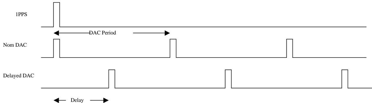
The delay shall be adjustable (from the VMEbus) over the entire range of the DAC clock period. The minimum step size for a 16384 Hz DAC clock period shall be one  $2^{22}$  Hz clock period. The minimum step size for the 2048 Hz DAC clock period shall be eight  $2^{22}$  Hz clock periods.
