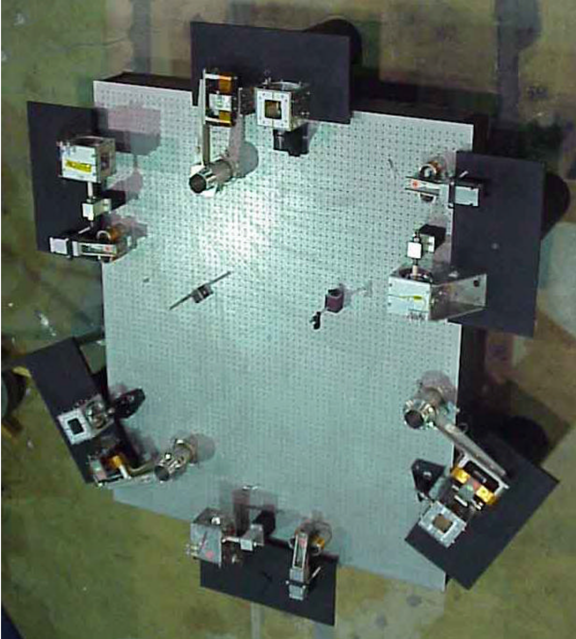
Figure 1 Eagle view of the HAM Active Internal Damping prototype. Visible at 60^\circ intervals are the alternated horizontal and vertical sensing/actuation doublets.
